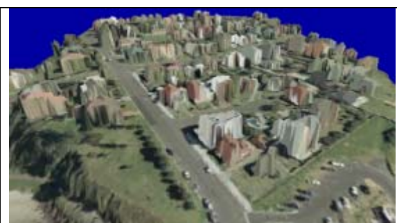
Fig. 16. Terrain with Houses and Draped Air Photo
