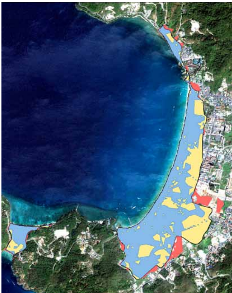
Figure 2. Simulated inundation using ANUGA versus observed inundation of the 2004 Indian Ocean Tsunami impact on Patong Beach. Blue regions indicate the areas where the predicted inundation matched the inundation survey. Red regions indicate areas where inundation was predicted but not observed, and yellow regions correspond to areas of observed inundation that were not predicted (Jakeman et al. 2010).
