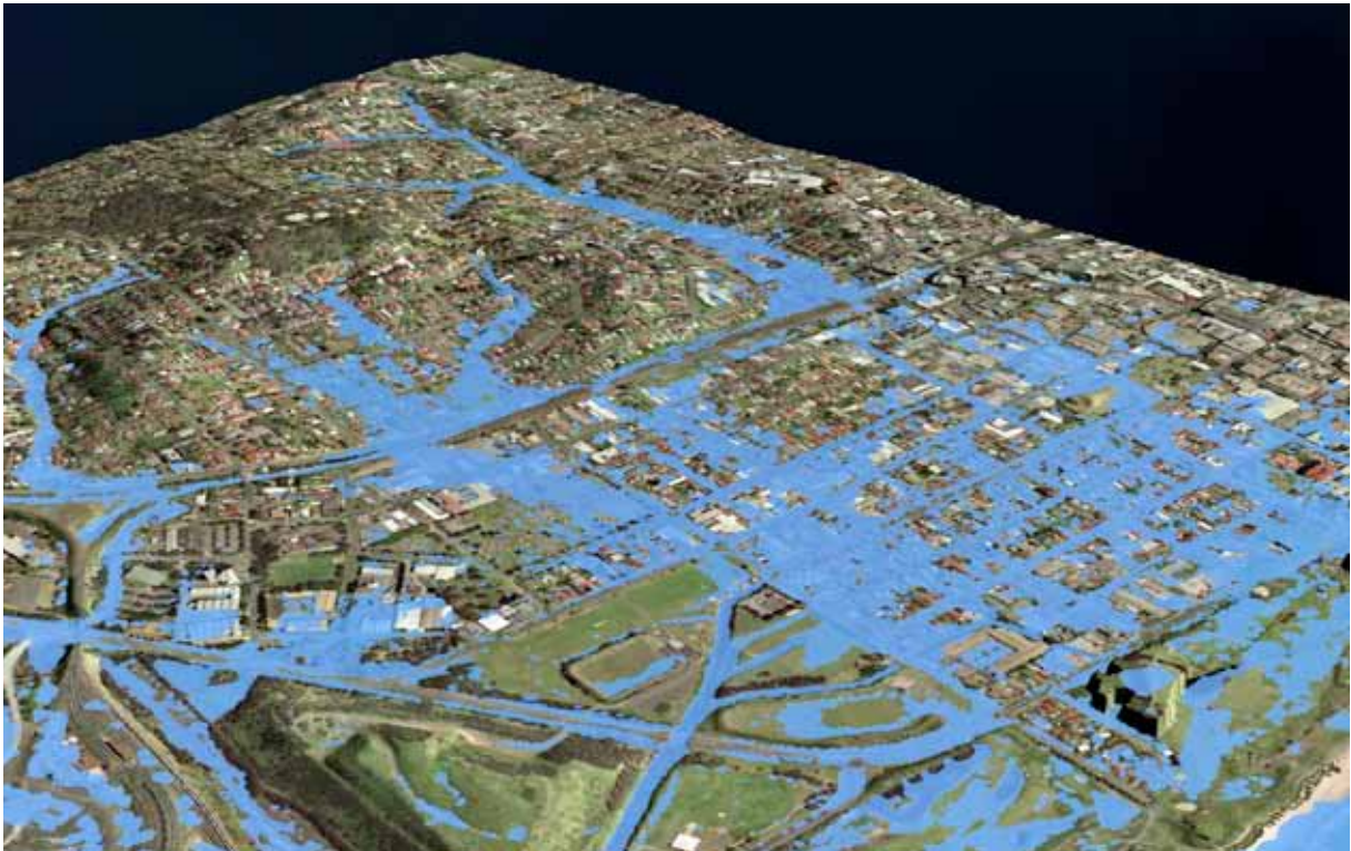
Figure 1. An example flood hazard scenario, simulated by ANUGA (P. Milevski, Wollongong City Council).
