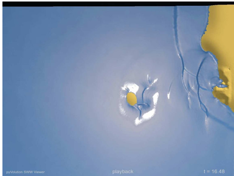
Fig. 3. Complex reflection patterns and run-up into Monai Valley simulated by ANUGA and visualised using our netcdf OSG viewer.
